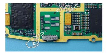
5. Tin one of the pads to fix the connector before soldering the following pins.
