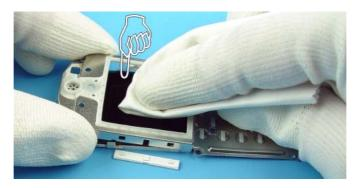
8. Always protect the LCD window with a protection foil to avoid dust and scratches.
