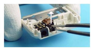
16. To remove the DC-jack, place tweezers between the spring contacts and under the jack. You'll need to use additional force to pull the jack upwards.
