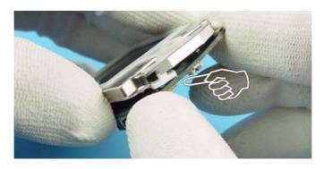
6. Separate the UI-shield from the system module carefully, Key dom is attached with adhesive tape, which must not be touched.
