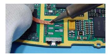
4. Note location markings to fit the connector precisely.
