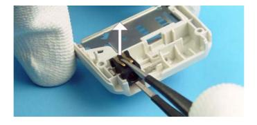
17. A straight bladed screwdriver can be used as a lever to remove the release spring.
