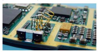
Note: You need a soldering iron with higher temperature when cleaning or soldering the ground pad.
