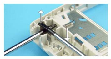
18. Release button will drop out when the B-cover is turned.
