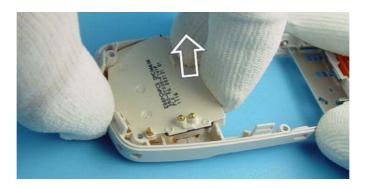
14. Use tweezers when removing the vibra motor.
